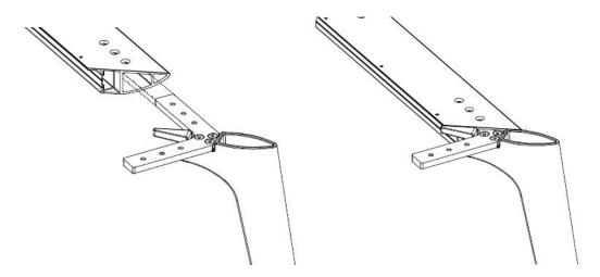
Step 11 Fix support rail to brace using three M6 x 16 countersunk socket head screws (SC090A) at each end of rail
